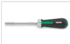
**STAHlwille ratcheting bit-holder** with easy direction changes (anticlockwise, clockwise and locked) by a quick twist of the switch ring and with an integrated storage space in the end of the handle.
